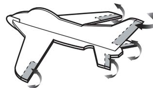
Have fun experimenting by bending wing and tail flaps slightly to alter flight patterns
